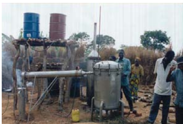
Picture 34. A small distilling unit for the processing of plant particles to obtain essential oil..
